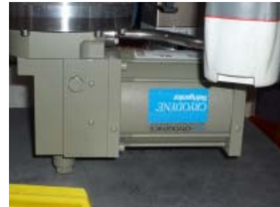
Gaseous helium cryogenic refrigerator
